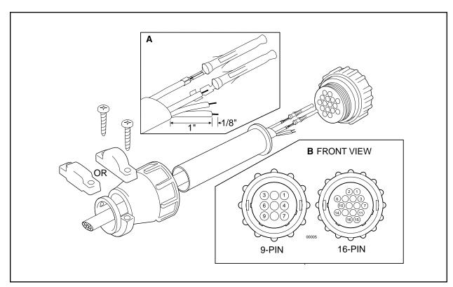
Figure 2. Connector Assembly
